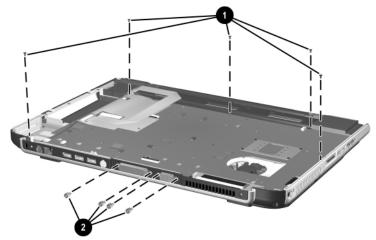
Removing the System Board Screws and Standoffs
